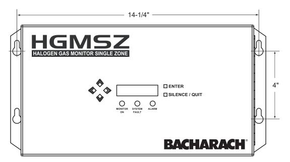
Hold the monitor flat against the mounting surface and allow it to slide down engaging the screw heads in the keyhole slots of the mounting brackets. Adjust the screws as necessary to hold the monitor securely against the mounting surface.
